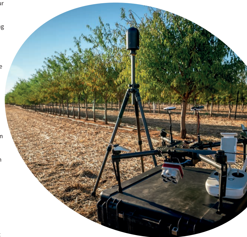
Research at the Mildura Smart Farm is utilising drones (foreground) and also LIDAR which is used in mapping orchard canopy, flowers, fruit and yield.
